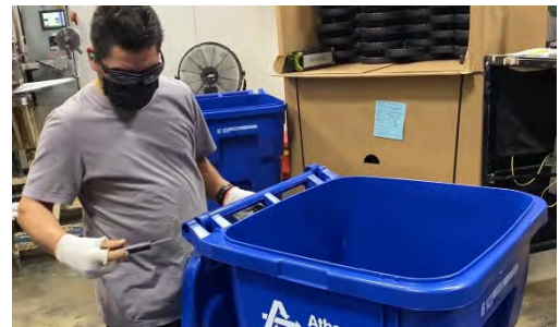
The RFID tag is inserted in the lid pin before the lid pin is secured to attach the cart lid to the body.
